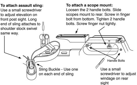
**Caution:** The finish on the bolts, safty switch bolt, front and rear sight screws and rivets heads is similar to gun blueing and will rust if not kept well oiled.
