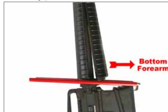
1B. Remove the factory lower forearm if using a vertical fore-grip.
