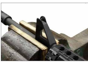
2. Clamp the upper receiver in a non-marring vise. Use only enough pressure to retain the upper during installation.
