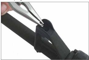
6. Place the **SIGHTLINK** detent with factory spring in the front sight assembly.
