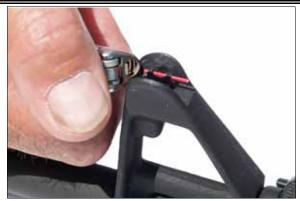
Insert the rod so that roughly  $^{1}/_{16}$ " protrudes from the rear (non-recessed end) of the blade, and touch a lighter (only for an instant) to the end of the rod to form the big bead. The longer the protrusion, the larger the bead that will form.
