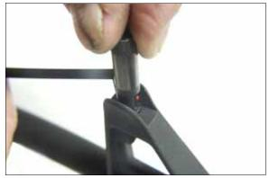
10. Depress the detent only far enough to clear the top blade while leaving the bottom post locked in place. Engaging <u>only</u> the top blade notches with the front sight tool, turn the **SIGHTLINK** blade so it faces forward, and then release the detent to lock the blade.
