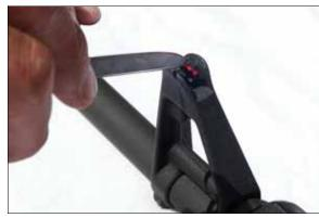
To replace a fiber-optic rod, first cut the old rod. Avoid scarring the *SIGHTLINK* blade.
