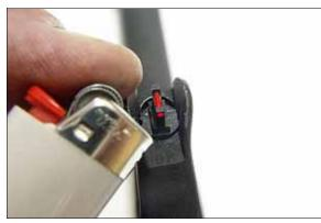
Touch a lighter to the front protrusion (only for an instant) to form the front bead inside the recess in the blade.
