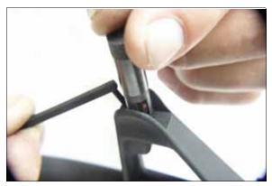
8. Depress the detent and thread the **SIGHTLINK** assembly into the sight housing
