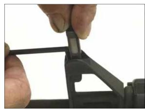
3. Place the front sight tool over the factory post. Use the detent bar to depress the factory detent and, while depressed, unscrew and remove the factory post.
