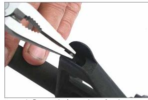
4. Remove the factory detent & spring.
