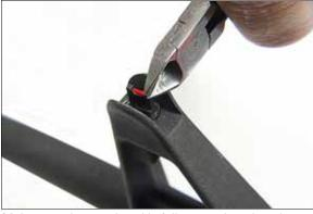
Make sure the rear bead is fully seated against the blade, and then trim the rod almost flush with the front (recessed end) of the blade, leaving not more than  $^{1}/_{32}$ " of rod protruding. Remember, the small bead should form inside the recess in the blade, and not protrude.
