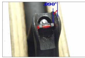
9. Initially set the blade depth at .090" below the top of the sight housing.
