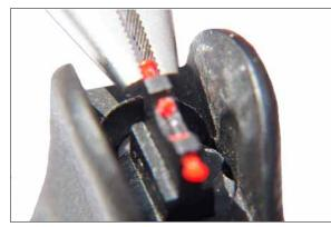
Remove both halves of the old blade.
